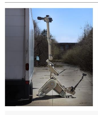
Kobra 725 provides unmatched strength, power, and payload support. The robot is designed to be a remote operational platform with a manipulator arm capable of lifting heavy loads. Kobra 725 is highly maneuverable in rough terrain and able to climb stairs. The state-of-the-art, IOP-compliant system allows for future payload expansion. Kobra 725 allows easy integration and deployment of a large range of accessories for EOD, CBRN/HazMat, breaching, and other applications.
