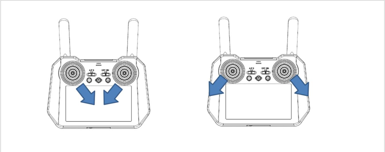
Pull both joysticks backward and in to start the motors. Push the left joystick forward to take off. Pull both joysticks back and apart to stop the motors.
