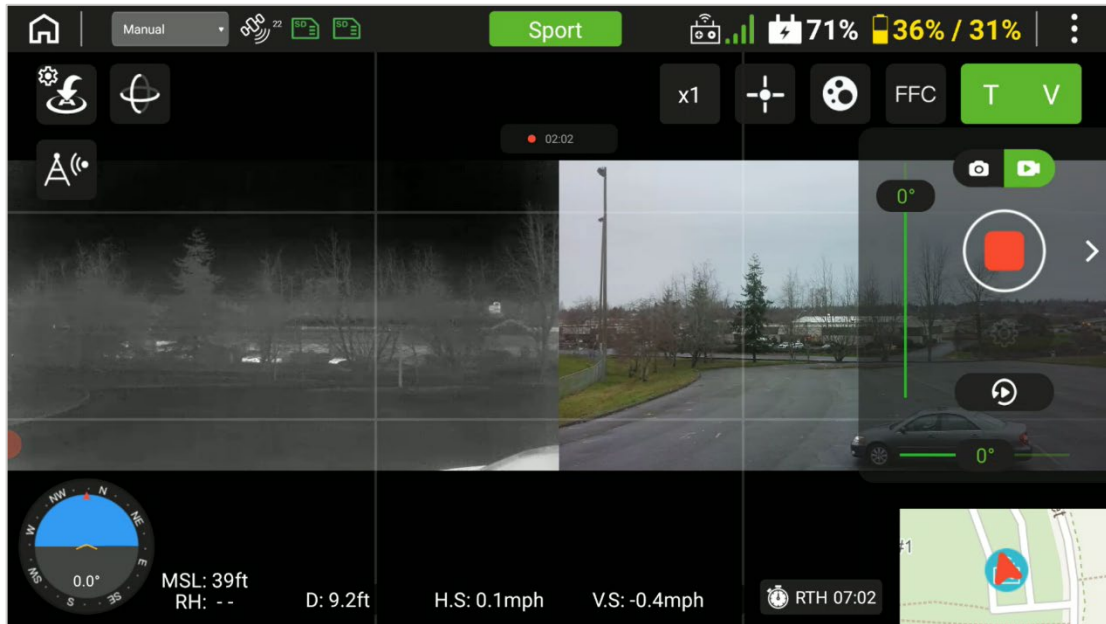
FIGURE 7.U THERMAL PLUS VISUAL DISPLAY
