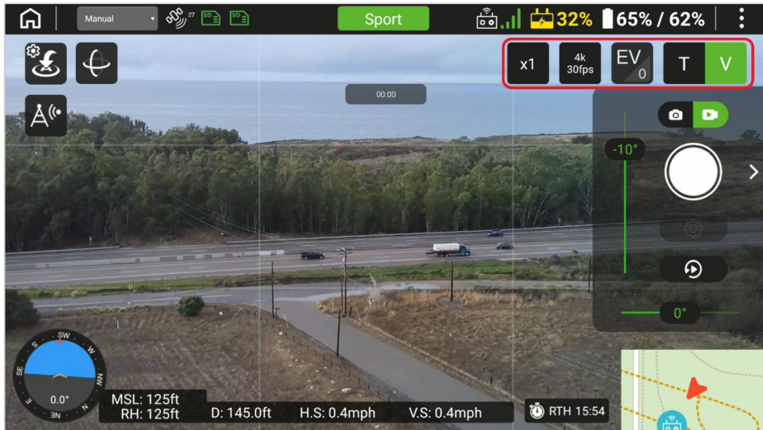
FIGURE 7.R VISIBLE CAMERA QUICK-ACCESS FEATURES
