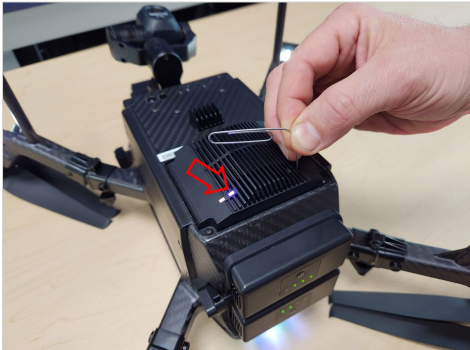
FIGURE 7.M PRESSING THE PAIR BUTTON (PAIRING LIGHT FLASHING)
