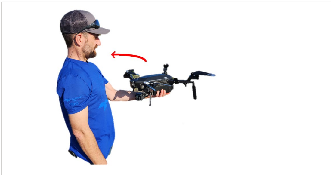
FIGURE 8.B COMPASS CALIBRATION STEP 2: HORIZONTAL ROTATION, LEVEL
