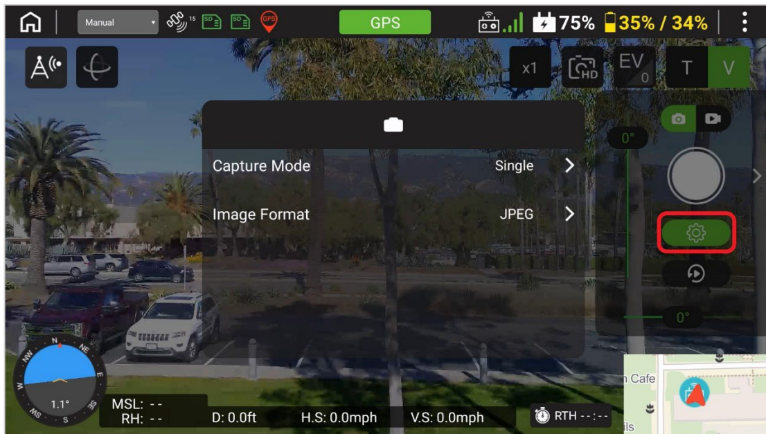
FIGURE 7.Y CAPTURE MODE AND IMAGE FORMAT SETTINGS FOR VISIBLE CAMERA
