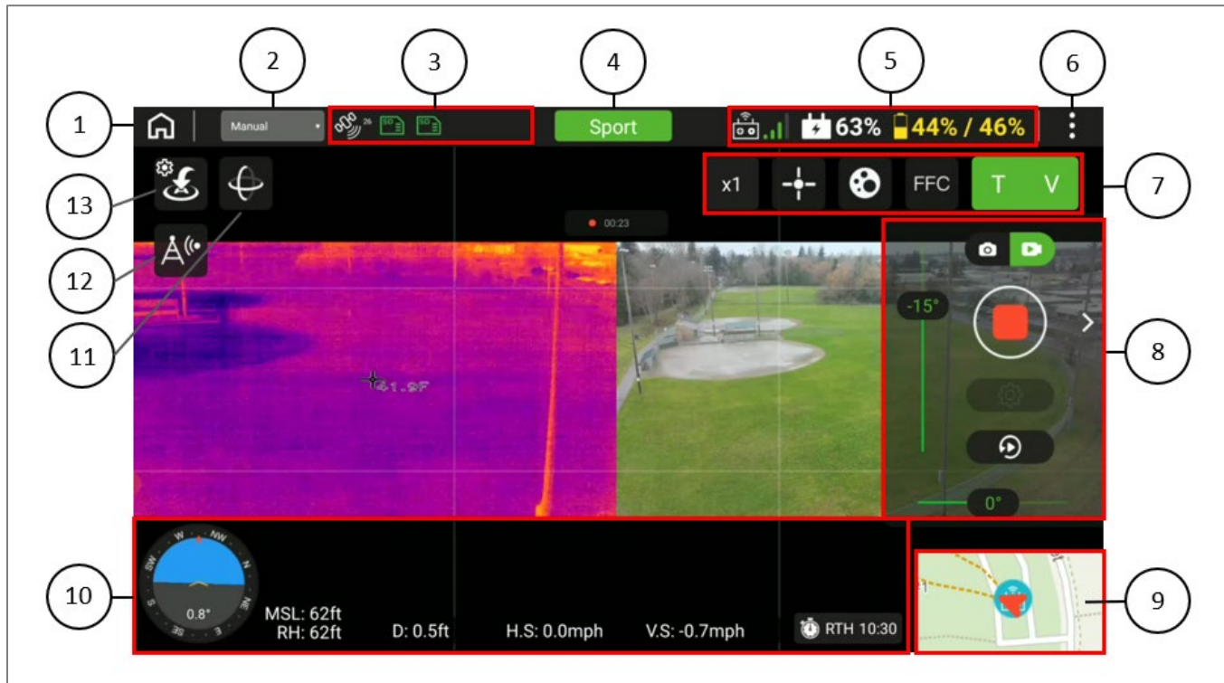
FIGURE 7.C GO FLY APP FLIGHT CONTROL SCREEN
