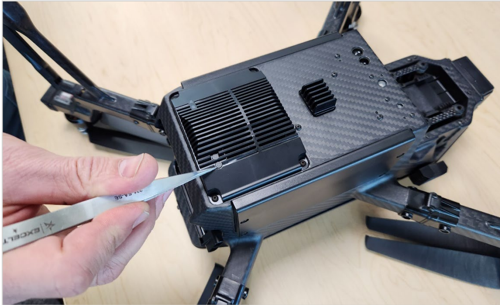
FIGURE 7.L PAIRING BUTTON COVER
