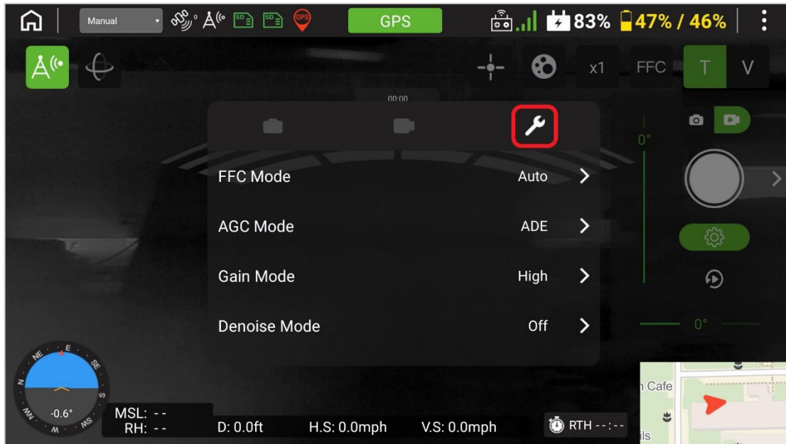
FIGURE 7.BB RADIOMETRIC ADJUSTMENTS FOR THERMAL CAMERA
