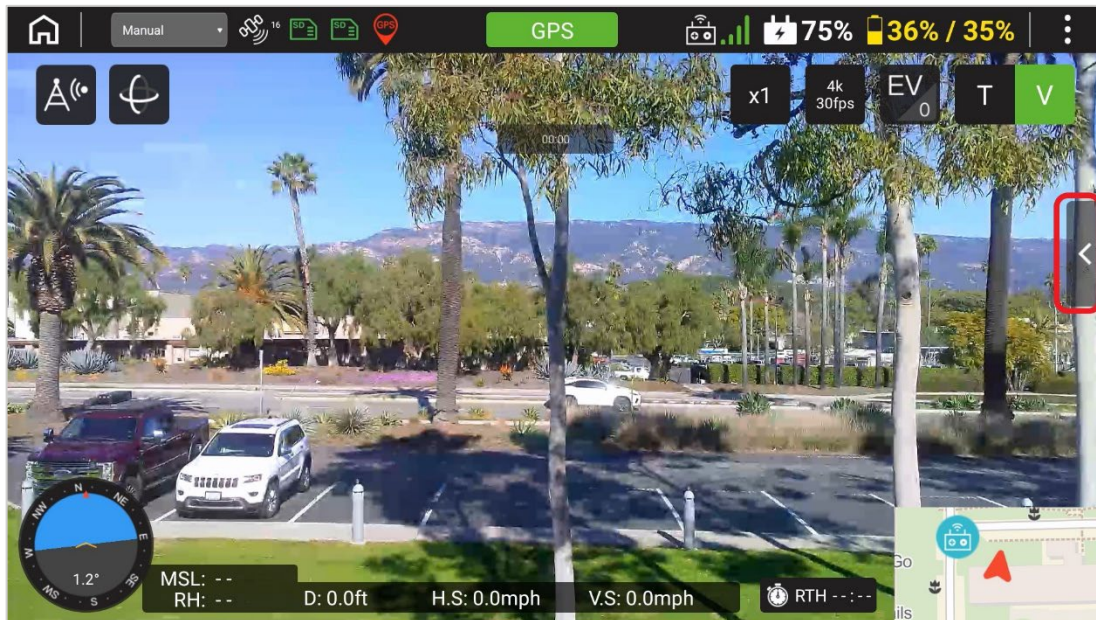
FIGURE 7.X BUTTON TO EXPOSE HIDDEN SHUTTER CONTROLS
