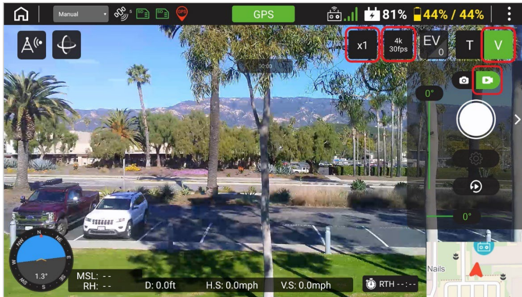
FIGURE 7.S THE VIDEO RESOLUTION ICON (VISIBLE LIGHT / VIDEO)
